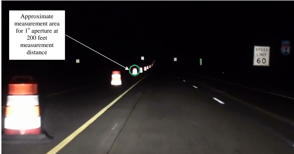
(a) Drums without steady burn warning lights, unlit freeway, prismatic sheeting
