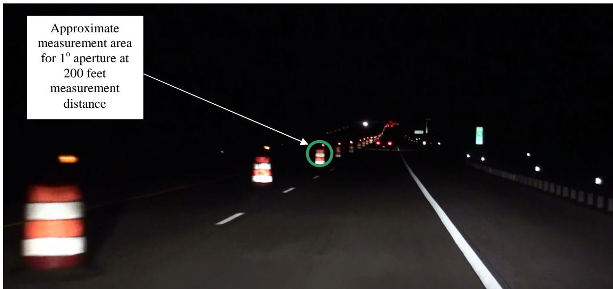
(b) Drums with steady burn warning lights, unlit freeway, high intensity sheeting
